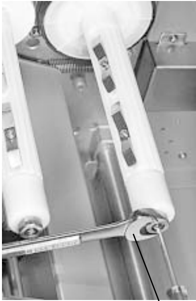
Fig. 6-41 USE 12mm OPEN END WRENCH AND PHILLIPS SCREW DRIVER TO REMOVE THE LOCKING SCREW AND ADJUSTMENT NUT
